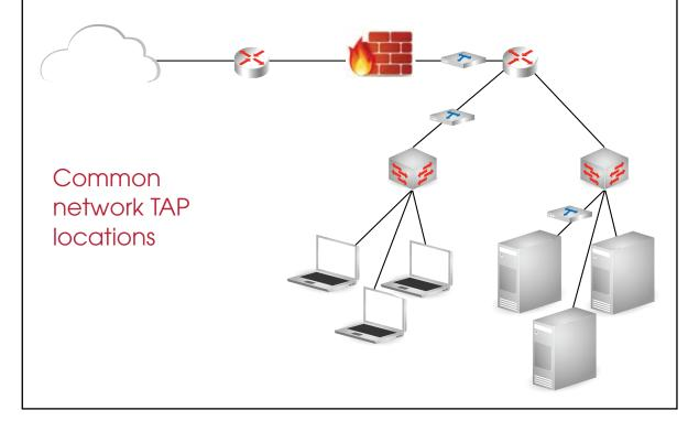
throughout the network. The passive nature of TAPs, ensure that network communication is maintained. Combining TAP outputs with the use of an aggregation device means greater visibility for the network probe.
